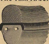
The accompanying cut shows rubber tire attached to wheel of a veh-
